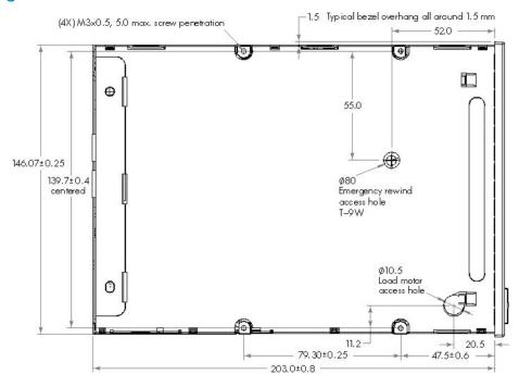
Figure 1 Full-height drives—plan
