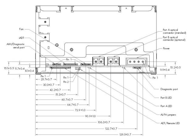
Figure 4 Full-height drives—rear view (Fibre Channel)
