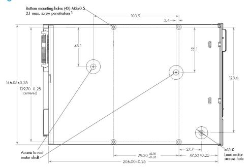
Figure 6 Half-height drives—plan
