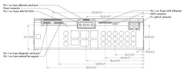
Figure 9 Half-height drives—rear view (Fibre Channel)
